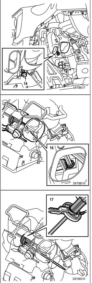
18 Grease all moveable surfaces from the left-hand side as shown in the illustration.
