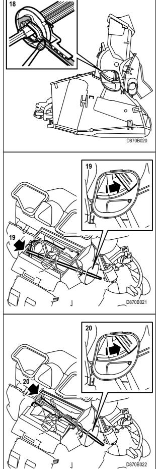
21 Grease the contact surface for the heating damper seal from the car's left-hand side.
